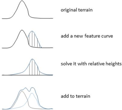
This works as long as there are no sharp features already existing right next to the new feature curve. If that is the case, as in the image above, adding the curves together produces unwanted results because of these inferences.
