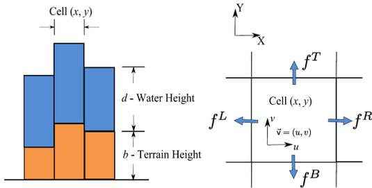
1) *Water increment:* Rainfall is simulated by sampling water drops over the terrain. The probability of each cell to 'emit' a water drop is equal to the moisture. The moisture map is initialized with the information created at the very beginning, in chapter IV-E. The user can edit this moisture value before starting the simulation. By using random rain drops instead of a global water increment, we add more randomness to the scene. A single raindrop erodes the terrain
