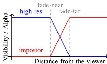
Figure 13: Blending between high resolution model and impostor
